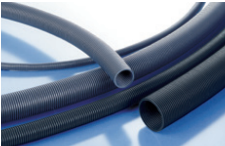
Conduits: PLR (PA6) and PCSL (PA12) conduits with high-grade, specially formulated polyamide. Very good flammability characteristics and mechanical performance.
